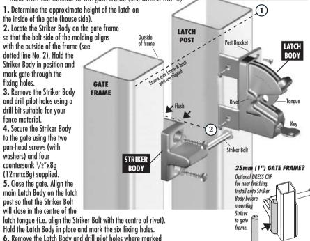
6. Remove the Latch Body and drill pilot holes where marked using the appropriate drill bit. Secure the Latch Body using the 1/2"x8g (12mmx8g) countersunk screws supplied.
